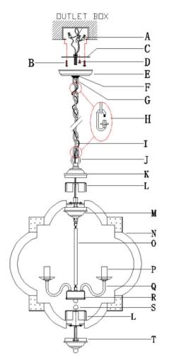
Step A1: Slip stem (O) over the wires and then thread it into the top of fixture loop (R). Slip Fixture body (M) over wires and then thread it onto the top of stem (O).
