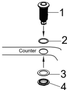
Mount the push button directly through a standard sink hole or drill a minimum 1 3/8" hole.
