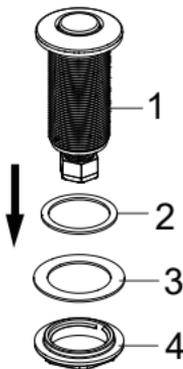
Remove the old air switch, clean the mounting surface. Remove the mounting nut (4), metal washer (3) and rubber washer (2) from the push button assembly (1).
