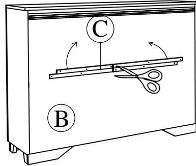
**STEP 2 :** Place the MIRROR FRAME (A) on the top of DRESSER (B), turn the MIRROR SUPPORT RAIL (C) upward at the back of DRESSER (B), then Tighten with CSK SCREW (D).
