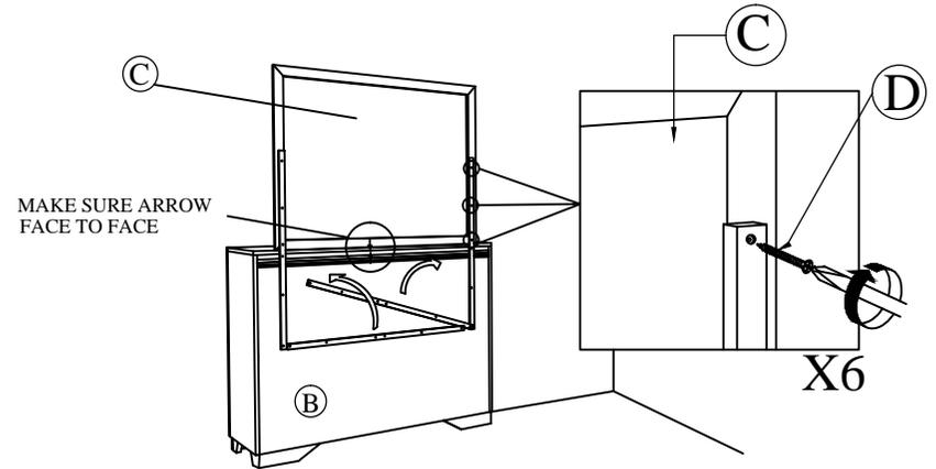
**STEP 3 :** Tighten the CSK Screw (D) as shown.
