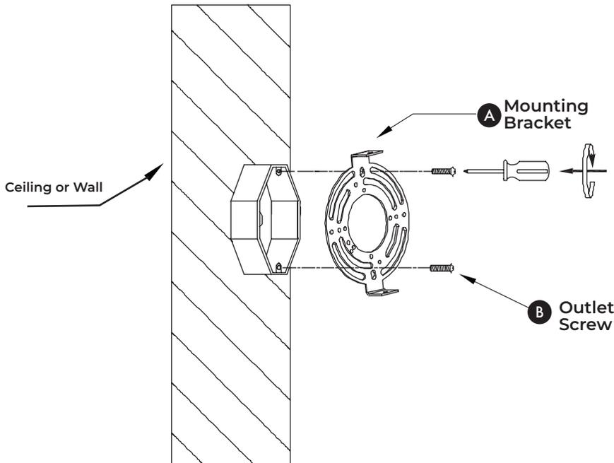
Secure Mounting Bracket (A) with Outlet Screws (B).
