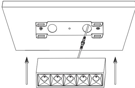
7. Connect the DC wire between fixture body and driver box. Place the DC wire into hole cutout in ceiling. Attach fixture body to mounting bracket firmly.
