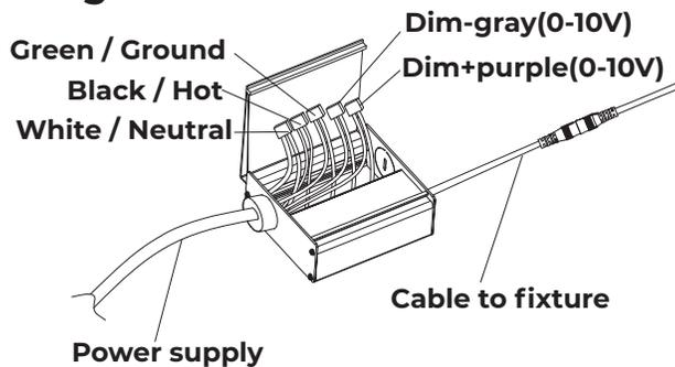
3. Connect fixture wires to building wires
