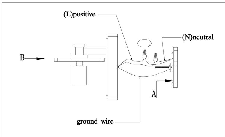
Step.2: Attach back plate to mounting bracket and tighten ball nuts so fixture meets wall. Caulk fixture where back plate meets the wall with silicone sealant. Leave a small gap at the bottom to allow moisture to escape.
