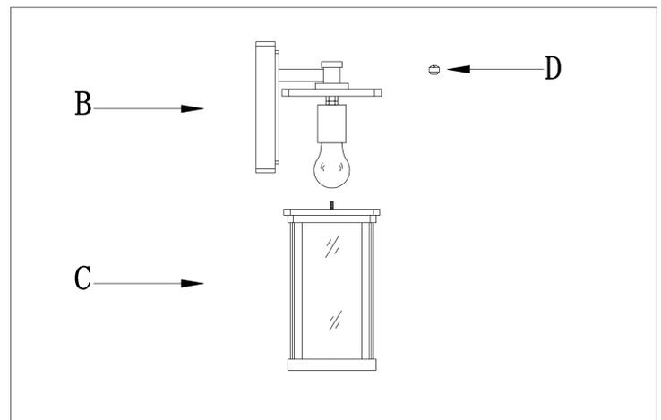
Step.4: Attach cage (C) to fixture , using ball nuts (D).
