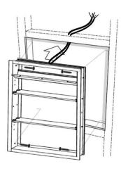
6. Insert and secure the cabinet; hardwire the power cord according to local electrical codes. You may hardwire both cables to the same power supply. Connect the wall switch to the white cable (Main) if one is used. A separate power supply is required for the Outlet (black cable).
