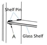
7. Insert Shelf Pins to desired height. Slide the Glass Shelf into position and tighten the plastic set screw (A) 8. Reinstall the Cover Plate and the Mirror Door(s)
