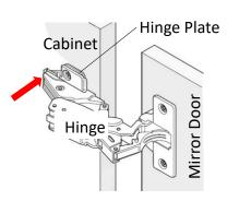
1. Unplug the cable from the Mirror Door to electrical enclosure. Remove the Mirror Door by pulling on the tab behind the Hinge to detach the hinge from the Hinge Plate. Remove the TOP hinge plate.
