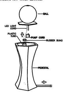
2. FILL RESERVOIR WITH APPROPRIATE AMOUNT OF WATER TO COMPLETELY SUBMERSE THE PUMP.
