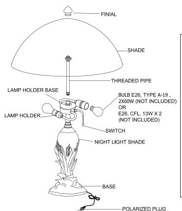
Instructions to install or replace the night light bulb: please unscrew the base cap to install or replace the night light bulb inside the night light shade.
