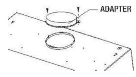
4. Measure the size of the outlet adapter relative to the cabinet and create an opening in the cabinet to let pass the outlet adapter and power cable. Make sure there is excess opening to accommodate electrical wires and hood exhaust. If you are installing the hood under the cabinet with a recessed bottom, it is advised to use a 4" wood fillers on both the sides.
