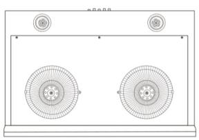
2. Remove the cover by carefully unscrewing the 3 screws as shown
