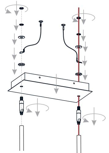
\* Make sure two swivels opening are in the same direction while assembling.
