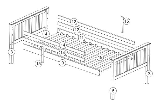
Loosen the appropriate hardware of the upper bunk so that the guardrails and leg assemblies are no longer connected to the bed assembly.
