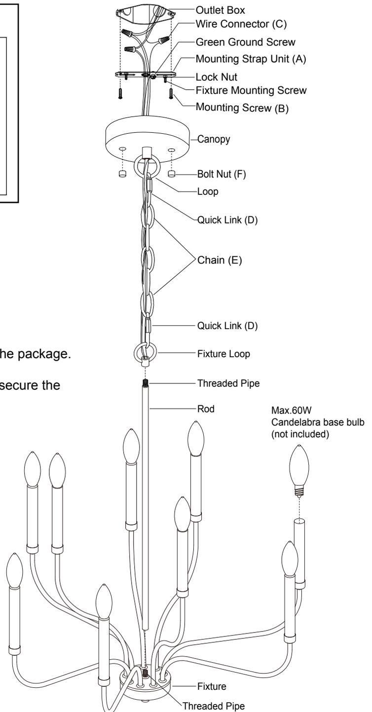
8. Attach the canopy to the mounting strap unit (A) and secure it with two bolt nuts (F) .
