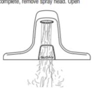
The OPTIMA Plus EBF-615 and EBF-650 Faucets are factory set to operate when hands are placed 4 to 5 inches (102 to 127 mm) from Sensor. This range should be satisfactory for most installations. If range adjustment is required, refer to the following range adjustment procedure.
