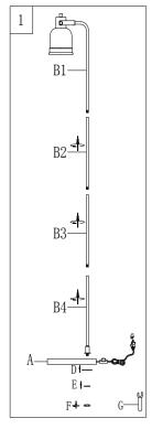
Step 1 Make sure all parts could be aligned before assemble Do not rotate lamp body too hard avoid base screw broken screw the Lamp body (B2) onto the Lamp body(B1); screw the Lamp body (B3) onto the Lamp body(B2); screw the Lamp body (B4) onto the Lamp body(B3); screw the Lamp base(A)onto the Lamp body(B4);
