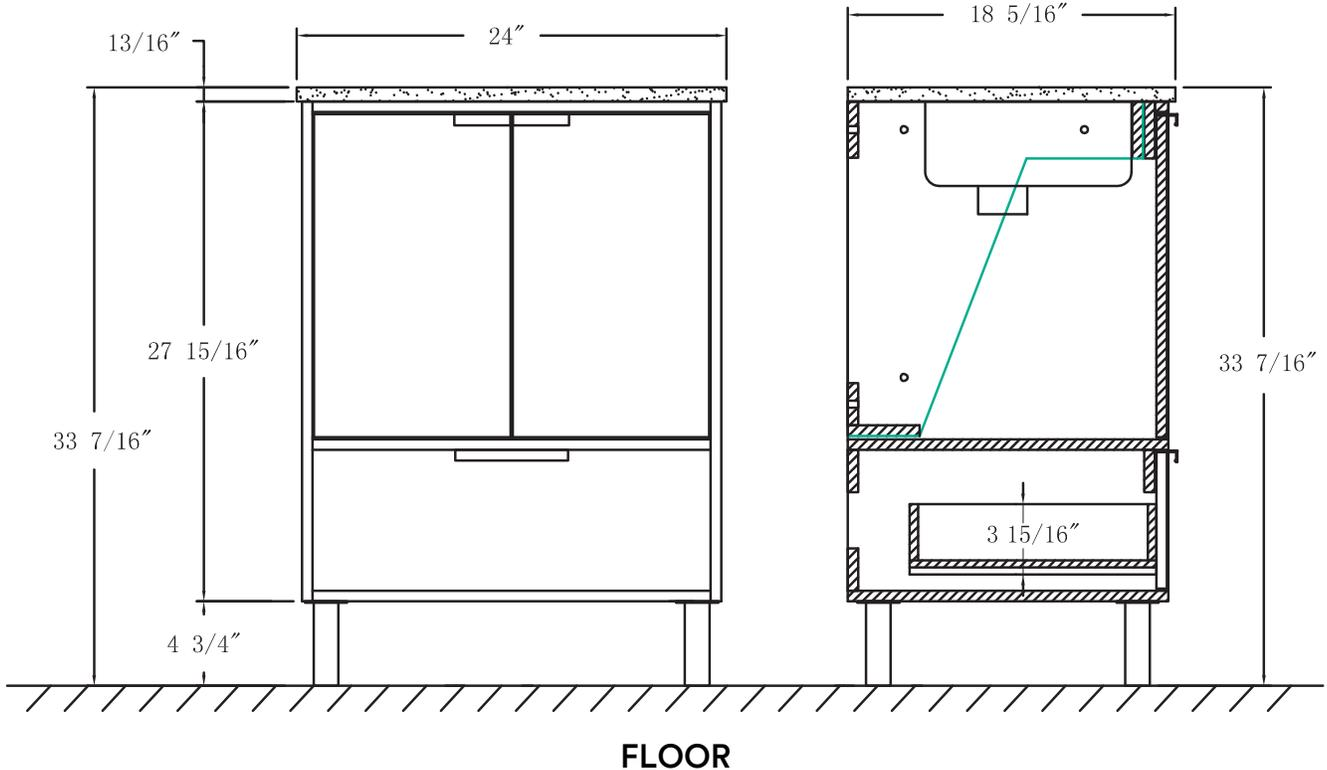
ATTENTION! DIMENSIONS MAY VARY BY UP TO  $\frac{1}{16}''$ . IT IS HIGHLY RECOMMENDED TO PULL ALL DIMENSIONS OF ACTUAL MODEL FOR INSTALLATION AND MEASURING PURPOSES.
