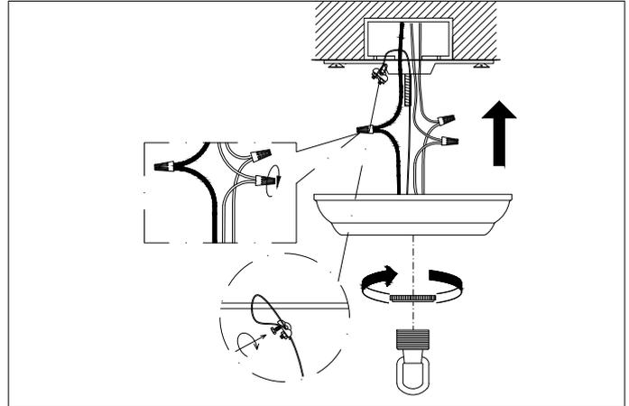
**2.** Connect the 3 power wires. The slick wires. The slick wire is the live wire, the coarse wire is the neutral wire, brass is the earth wire. Connect the wire lock.
