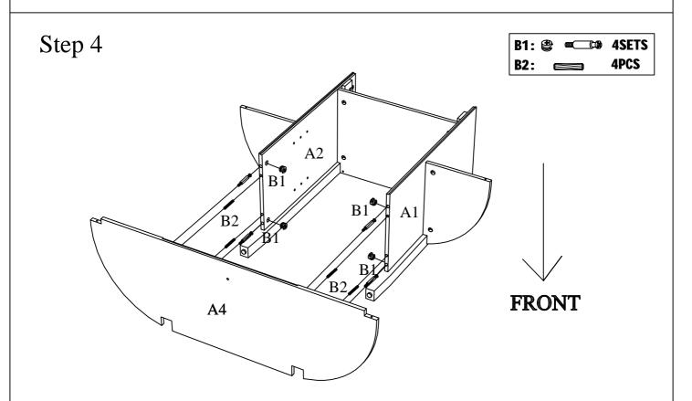
Assemble Bottom Panel A4 to Dividers A1&A2 using Wood Dowels B2 & Camlocks B1.
