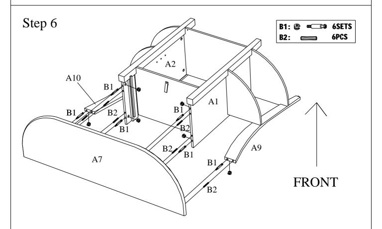
Assemble Top Panel A7 to Legs A9&A10 and Dividers A1&A2 using Wood Dowels B2 and Camlocks B1
