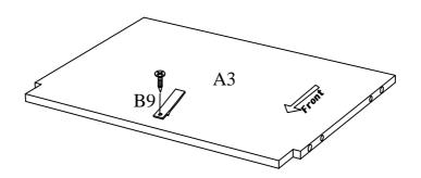
Attach Stopper B9 to Center Shelf A3 using including screws.(Hole is pre-drilled)
