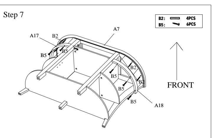
Assemble Aprons A17&A18 to Top Panel A7 using Wood Dowels B2 and Screws B5. Note:Holes are pre-drilled.
