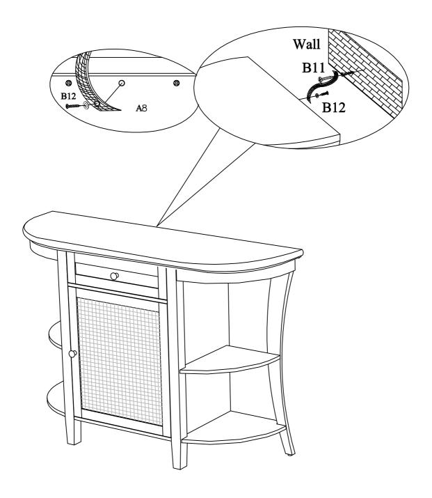
For your safety, please attach this unit to the wall by Anchor with Screw B11 and Anti-tip kit B12.
