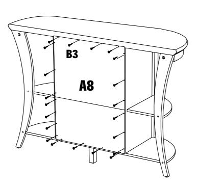
Attach Back Panels A8 to the back of this unit using Screws B3.
