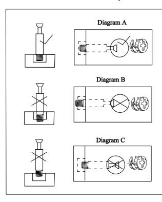
1. Insert cam screw into hole as shown in diagram A.
