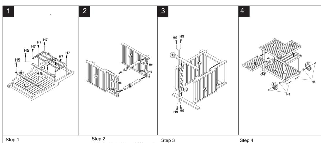
Use (H7) to attach (H4) to (C), and use (H5) to attach (H1) to (C), use allen key (H10) to tighten (H7) and (H5).
