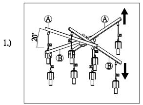
Step.1: Adjust the lamp body(F), adjust the tube(A) to up 20 degree and adjust the tube(B) to down 20 degree after remove package
