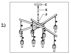
Step.2: Carefully remove packaging from fixture.Run wire through stems (E) and combine stem lengths to meet desired mounting height. Then attach canopy (C) to fixture.
