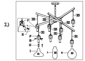
Step.3: Insert the G9 bulbs one by one Attached the glass(B1, B2, B3) to yoke and secured with lock screw(H)
