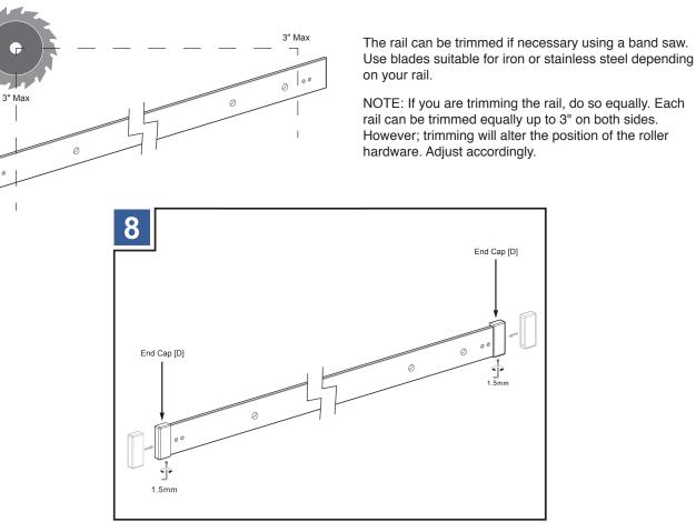
Once cut, add the end caps [D] to the ends of the rail and secure with a set screw.
