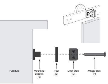
Install the rail, mounting brackets [E], and door stops [C].
