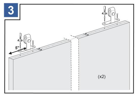
Drill holes into the doors as indicated. Attach the door roller [A].
