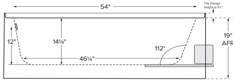
This tub model features a 19" skirt height that allows for above floor rough-in.
