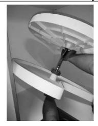
From the top slide one (1) Shelf Assembly, the other Shelf Support and then the other Shelf Assembly onto the Pole Assembly as shown. Slide bottom of Pole Assembly into the lower mounting support.
