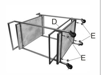
Attach bottom shelf (D)to be metal legs and fasten by  $\operatorname{nuts}(E)$ , and using the  $\operatorname{wrench}(F)$ .
