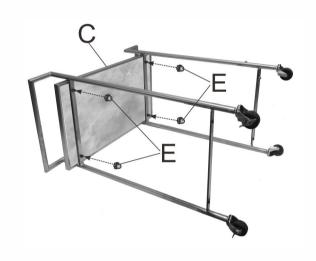
Attach top shelf (C)to be metal legs and fasten by  $\operatorname{nuts}(E)$ , and using the  $\operatorname{wrench}(F)$ .
