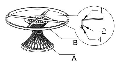
Connect Stainless steel pillar (B) with Table top frame (C) by Screw (2), Tighten
