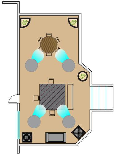
The unit must be placed on a level surface to operate correctly. Units create an oval shaped air pattern. Obstacles such as racks and workbenches may interfere with the air flow. An attempt should be made to locate the unit in such a manner that interruption of the air pattern is held to a minimum. Multiple units may be required to cover larger areas.
