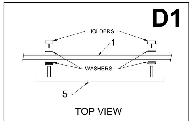
**E. INSTALLING THE DOOR BOTTOM SEAL STRIP**
