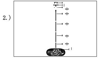
Step. 2: Run wire through stems(B) and combine stem lengths to meet desired mounting height.
