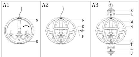
Step A1: Open the Wood bending (N) and arm (R) to equal.
