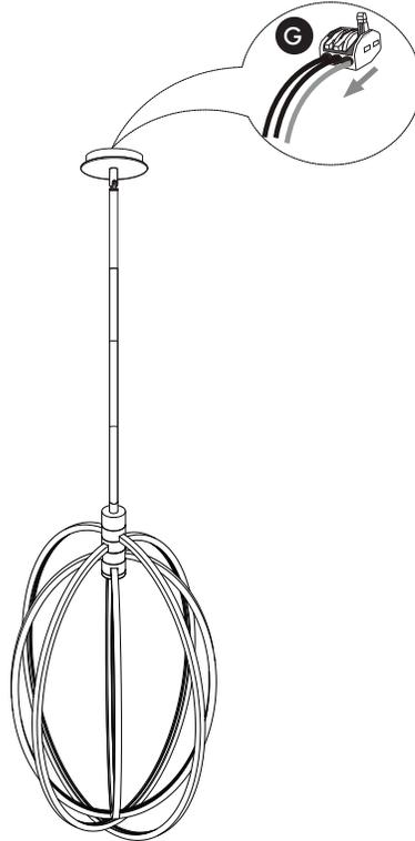
Remove wire from wire connector (G).
