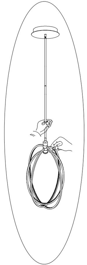
**Installer Tip (3): Separate the rings one by one using both hands. DO NOT USE EXCESSIVE FORCE.**
