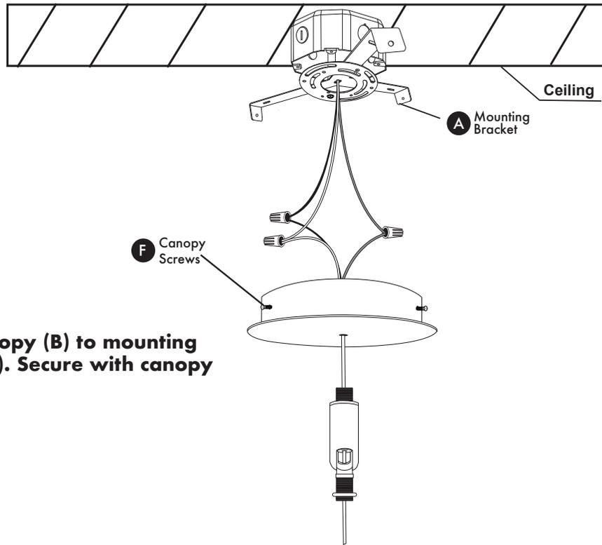
Attach canopy (B) to mounting bracket (A). Secure with canopy screws (F).
