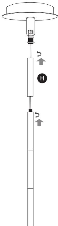
Secure and tighten additional down rod (H).
