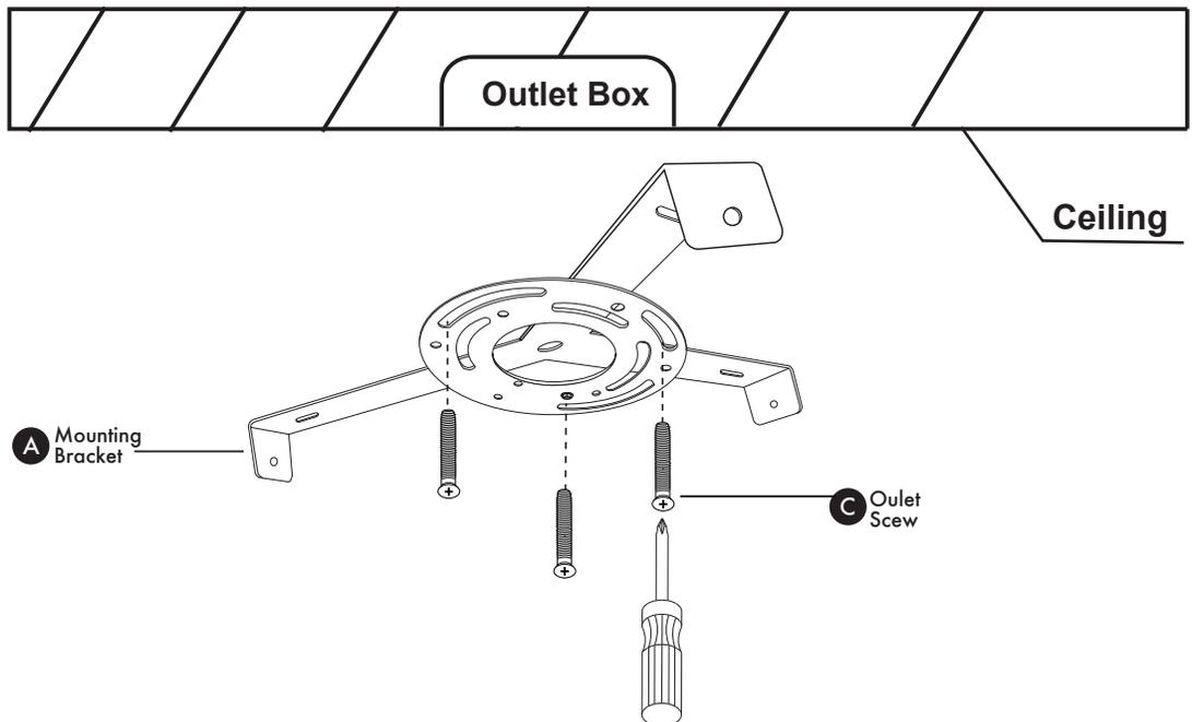
Attach mounting bracket (A) to outlet box. Secure with outlet screws (C).
