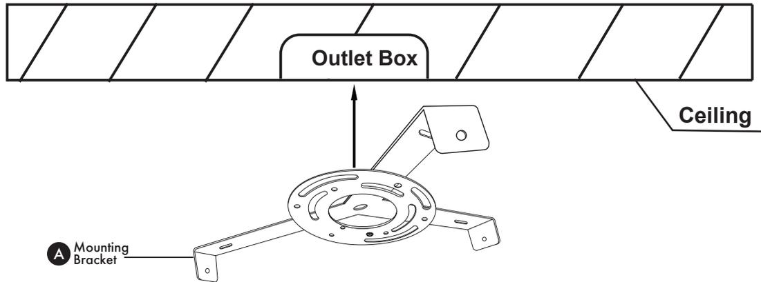
Align mounting bracket (A) with outlet box.
