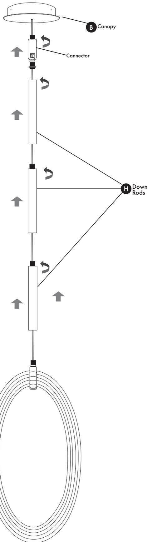
**Connect down rods (H) together and tighten by hand. Connect attached down rods (H) to connector and secure into canopy (B).**
