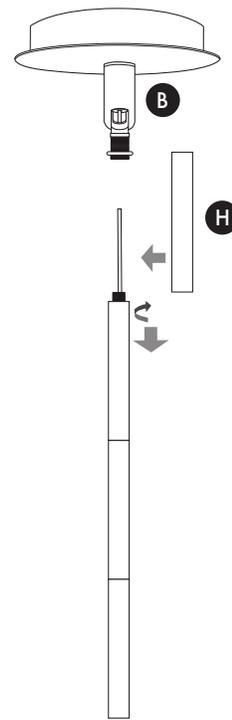
1. Unscrew down rod (H) from connector (B).
