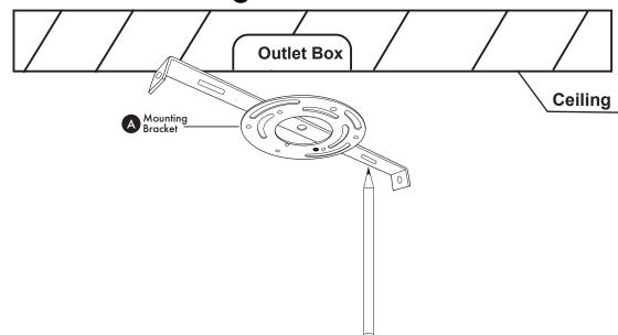
Raise mounting bracket (A) to the ceiling. Mark location for the plastic anchors (B). Use drill holes for plastic anchors (B). Insert plastic anchors (B) into hole.
