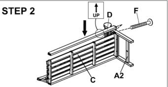
Attach apron (D) onto seat (C) and left side frame (A2) and secure using 2" bolt (F) as shown.
