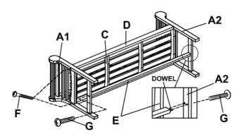
Attach right side frame (A1) into back support and apron and secure 2" bolts (F).
