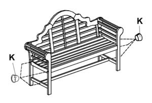
Tapping in the wooden caps (K) to cover bolts head using rubber mallet.
