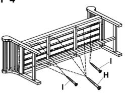
Secure the seat (C) using 1 1/4" screws (H) into back support and apron and 1" screws (I) into side frames.
