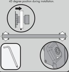
Place Grab Bar in desired position on wall, being sure that there is sufficient blocking within the wall. Level if desired. Mark four (X4) holes from each Wall Plate onto wall with pencil.
