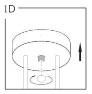
Lining up threads on crossbar with hole in backplate, attach fixture to junction box using cap nut. Be sure to carefully tuck wires into backplate while attaching.
