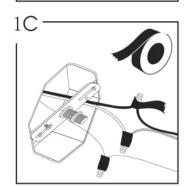
Tape wires and wire nuts together using electrical tape.
