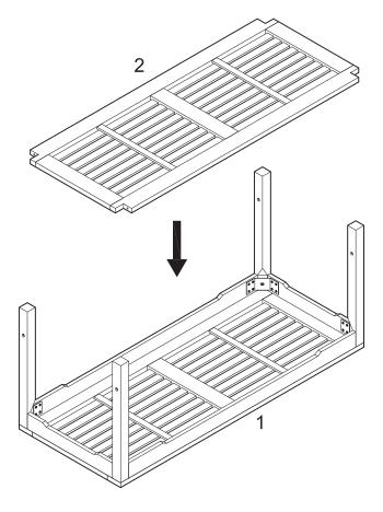
Carefully slide shelf (2) into place. (Shelf (2) will align with the pre-drilled holes of the table legs.)
