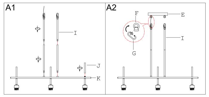
Step A1 » 1) Carefully pass the fixture wires through one side of tubes (I) and loops (F).
