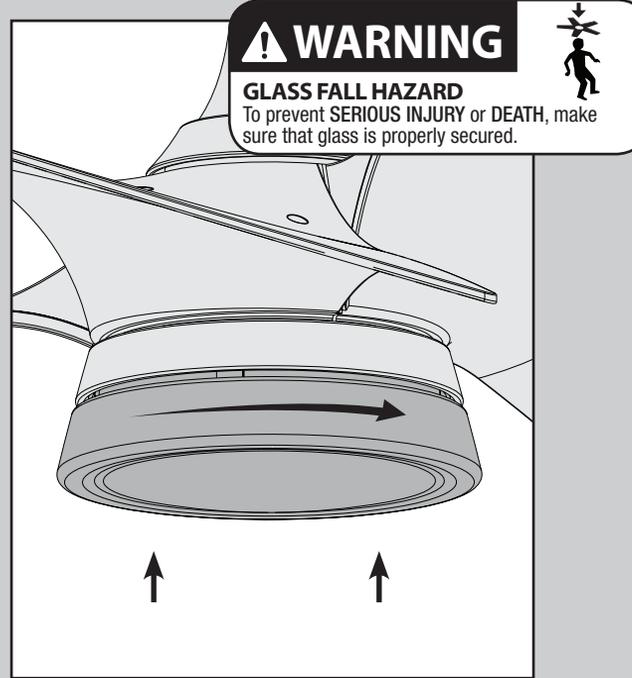
Carefully lift the globe up inside the LED assembly as far as it will go, then rotate the globe clockwise until it is held tightly in place by the tabs.
