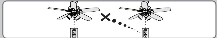
If a transmitter is mistakenly operating a fan, you need to “unpair” the transmitter from that fan’s receiver. The “unpairing” procedure is the same as the pairing procedure.
