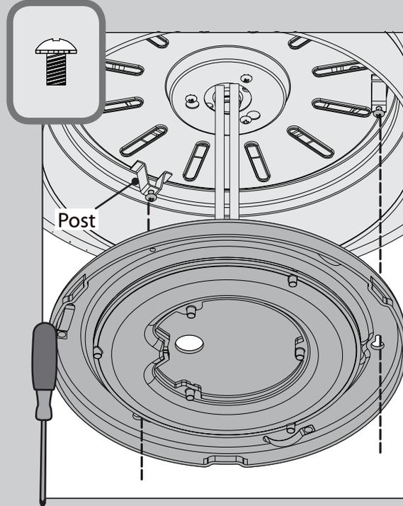
⊗ Screw two LED assembly screws, found in the ≡ hardware bag, halfway into two of the posts in the upper switch housing. Push any excess wiring into the switch housing, then wrap the keyhole slots in the LED assembly around the screws and twist clockwise.
