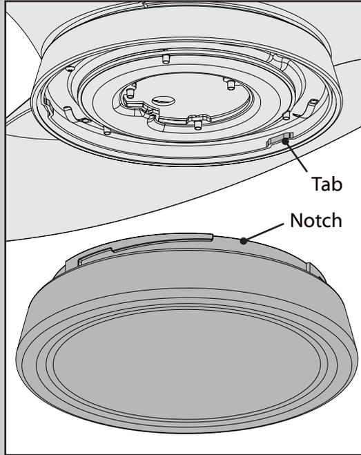
Position the notches in the outer rim of the globe so they line up with the three tabs on the inside rim of the LED assembly.
