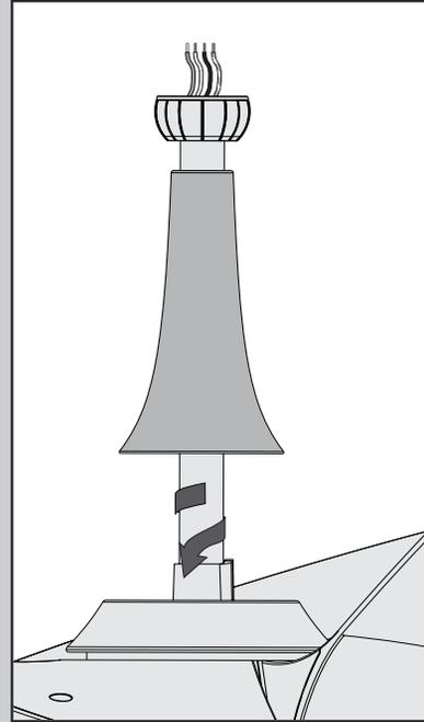
Slide the adapter cover over the downrod, then hand tighten the downrod (at least 4-5 full turns) until it stops.
