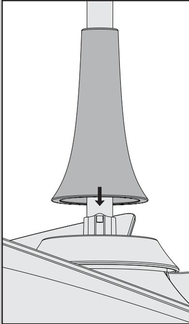
Lower the adapter cover until it rests on top of the motor housing.
