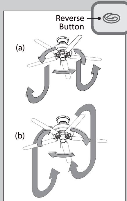
The reverse button on the wall control changes the air flow pattern. **In warm weather**, use (a) downward air flow pattern. **In cold weather**, use (b) upward air flow pattern.
