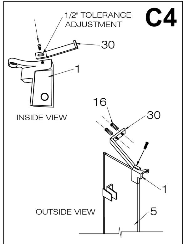
5. Screw the structural arm into the wall with 1 1/8" phillips screws (#15) making sure it is firm and plum to the wall and keeping the front fixed panel at a 90° angle.
