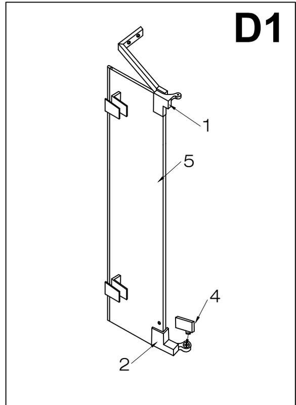
2. One installer manually inserts the convex portion of the turning hinge (#3) into the concave portion of the turning hinge base (#1) and holds the position. The hinges should be turned to a slightly open position.
