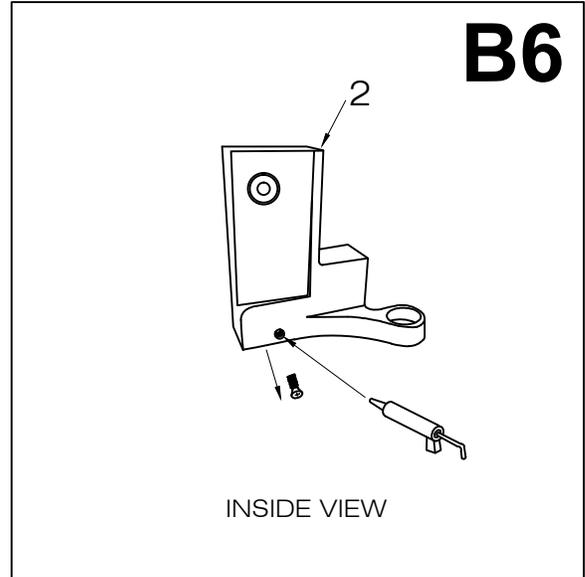
7. Mount the turning hinge base (#1) to the upper corner of the front fixed panel, cover the plate and tighten the screw (supplied) from inside the shower.
