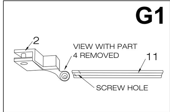
2. Place the left threshold end cup (#28) on the left end of the door threshold (#11). Then carefully align the door threshold and threshold end cup under the door panel. The threshold end cup should be placed against the turning point of the hinge base mirrored, while the other end of threshold should be placed against the wall.
