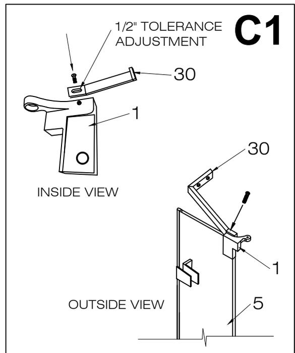
2. Mark two holes on the wall for the mounting screws for the structural arm (#30).
