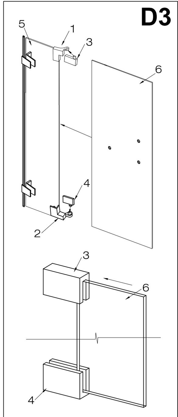
4. Tighten three screws (supplied) on both turning hinges from inside the shower, respectively, making sure the door panel is tightly secured by these two hinges and level.
