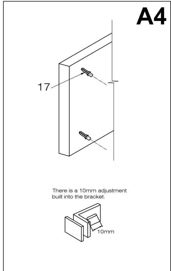
5. Replace the front fixed panel. Screw into the wall with 1 5/8" hex screws (#13).
