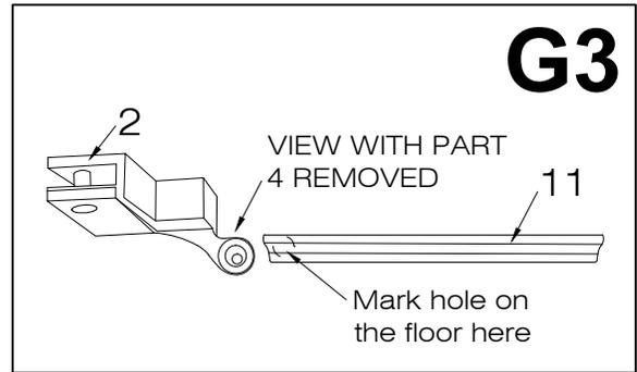
4. Remove the door threshold and drill hole into the floor. Insert plastic anchor (#16) into the hole.
