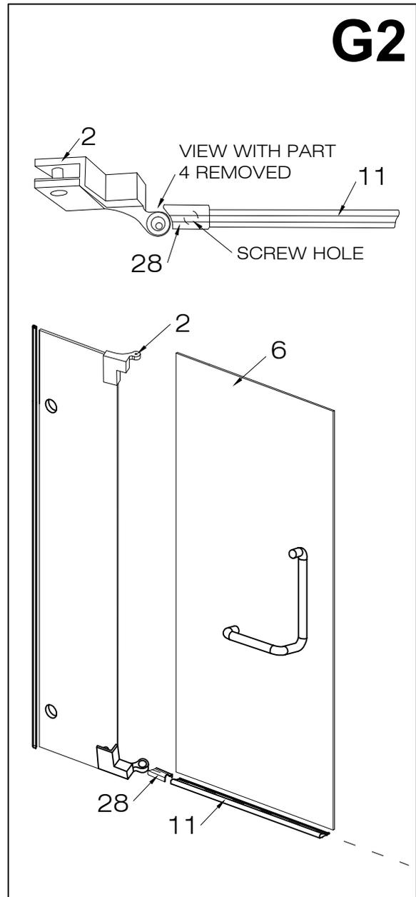
3. Remove the threshold end cup and mark a hole on the floor for the threshold screw.
