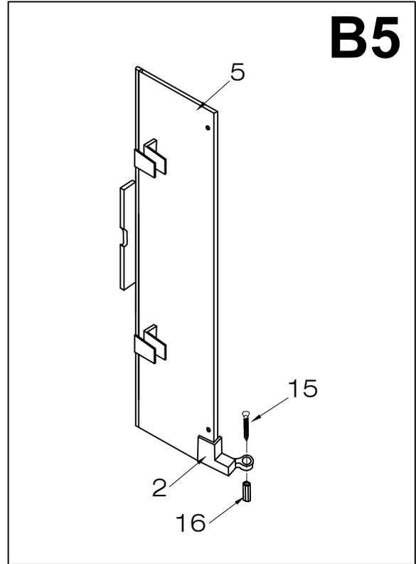
6. Remove the screw that connects the structural arm on the floor mount portion of part (#2). Removing this is to prevent personal injury, silicone the void to prevent water entry.
