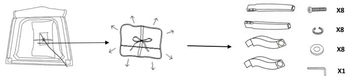
Step 2.Using bolts (H1), lock washers (H2), flat washers (H3), connect legs(P1,P2,P3) to Chair (P4). Tighten bolts (H1) with Allen Wrench (H4).
