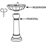
**2.** Feed the pump and LED light cables through the plastic tube in the reservoir, and through the channel on bottom of the pedestal.
