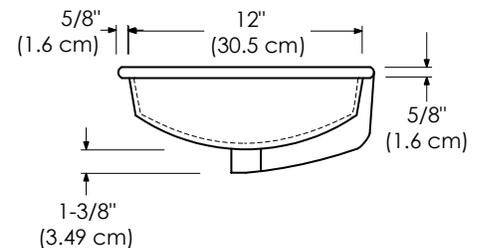
By IAPMO, ceramic lavatory warpage is defective only if warpage of flat slab out of horizontal plane exceeds 6.3 mm/m (0.25 in/ft) on all sizes OR warpage on back of lavatories that are attached to the wall exceeds 3 mm (0.13 in).
