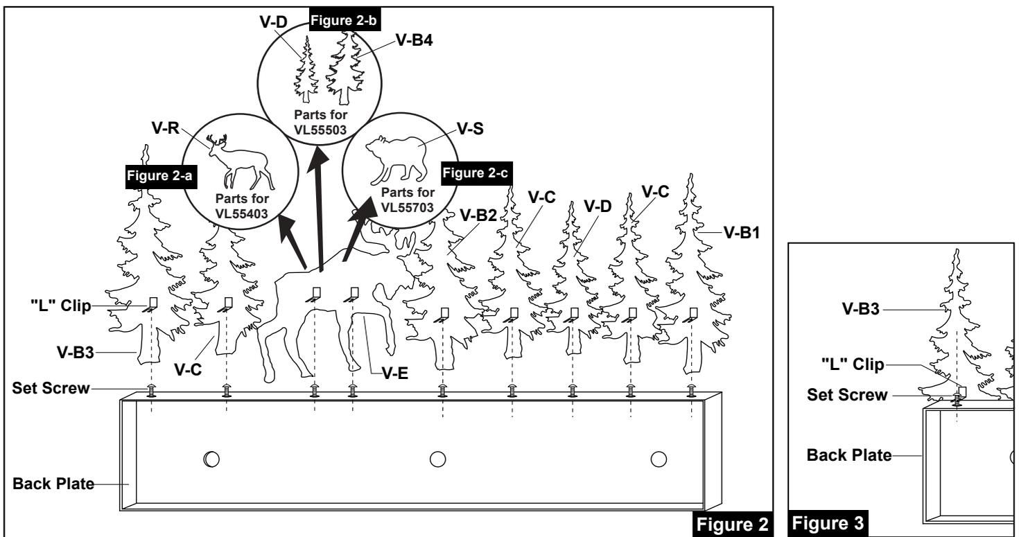
3. Install the silhouettes onto the back plate.
