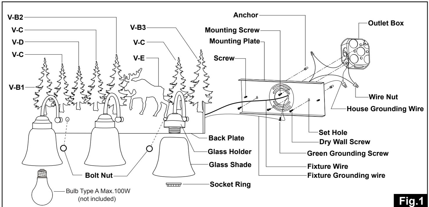
1. Unscrew two bolt nuts, and remove the mounting plate from the back plate.
