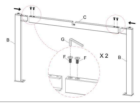
Assemble the Lower Cross Bar (D) to the Leg Post (B), then using the Bolt (F) by Allen Wrench (G).
