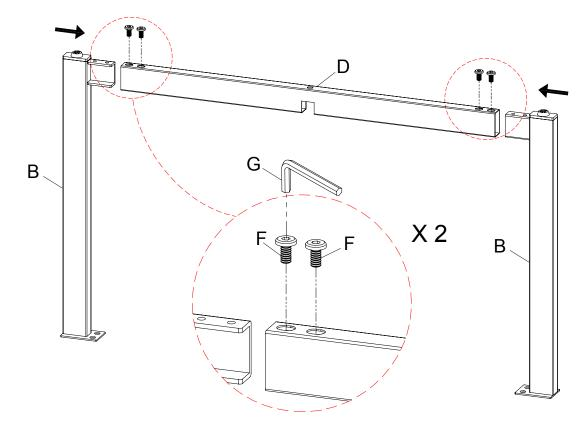
\*\*\*Do not tighten screws & bolts until the entire unit is completely assembled.
