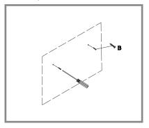
**Step 04:** Use screwdriver screw the screw into the expansion screw, tighten. And then leave a distance of about 5MM from the wall.
