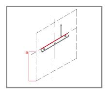
**Step 02:** Mark the punching position on the wall with a pencil. use level gauge make sure the hole at the same level.
