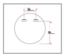
**Step 01:** Check the wall.Make sure that the wall is bearing walls that can support the Mirror's weight. Measure the width and height of the mirror back holes/hocks distance with a tape measure.
