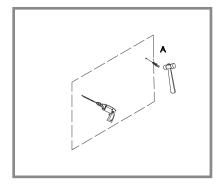
**Step 03:** Use impact drill punch holes in the marked center (6-8MM drill bit), the drilling depth is about 5CM. Use a hammer to drive the expansion screw into the drilled hote.
