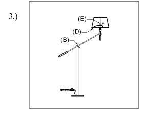
Step 3: Remove the socket ring (E) from fixture (B). Attach shade (D) and secure using socket ring (E).
