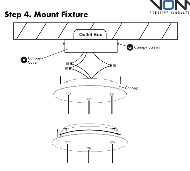
Attach canopy to canopy cover (A). Twist canopy to lock fixture in place. Secure canopy with canopy screws (G).
