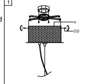
2.Please Screw part (A) and (C) onto the 2 lampbody (B)
