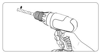
Drill holes in using 1/4" drillbit.
