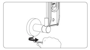
Use the provided allen wrench to adjust the set screw to lock into place with the mounting bracket.
