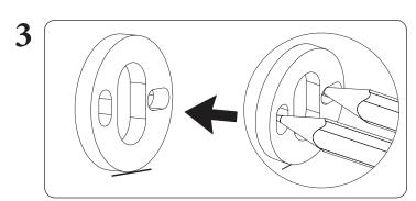
Place mounting plate on the wall and mark position of the holes in the mounting plate.
