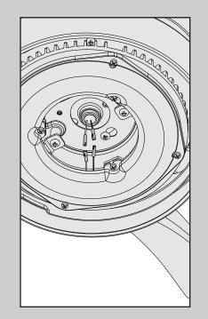
Connect the white wire from the fan to the white wire from the light kit. Then, connect the blue wire from the fan to the black wire from the light kit. Lift the globe and align the notches in the globe with the tabs in the light kit. Attach the globe by lifting and twisting clockwise until it rests firmly in place.
