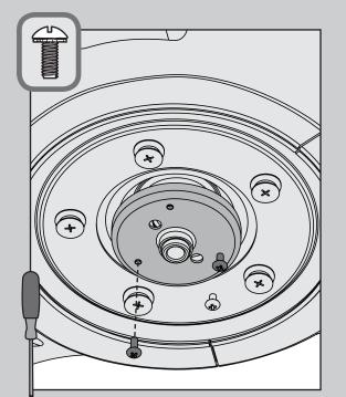
Screw two housing assembly screws from the ≡ hardware bag halfway into the motor housing. It does not matter which two screw holes you choose.
