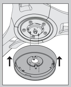
Wrap keyhole slots around the screws and twist counterclockwise.
