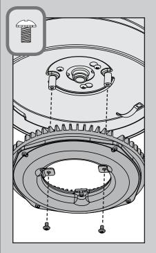
Raise the LED assembly to the posts in the housing. Attach the LED assembly using the LED assembly screws found in the ■ hardware bag.
