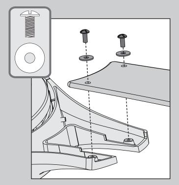
Put the blade washers found in the ■ hardware bag onto the blade screws found in the ▲ hardware bag. Then install the blade screws to secure each blade to a blade iron.
