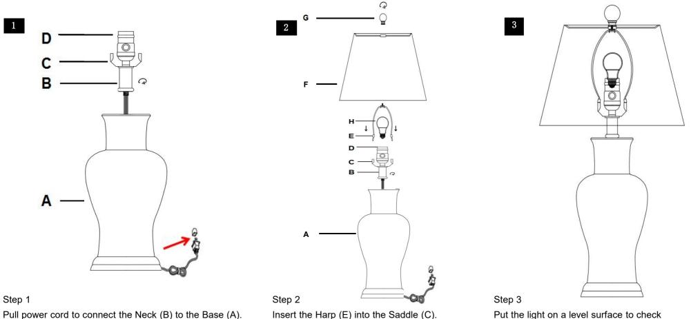
Pull power cord to connect the Neck (B) to the Base (A). Screw the Neck (B) onto the Lamp base (A) Be careful not to twist the power cord and tighten securely Insert the Harp (E) into the Saddle (C). Put the shade(F) on the Harp(E), then tighten the Finial (G)into the Harp (E) Insert the bulb(H) into the socket(D).
